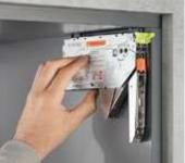
Choose between two symmetrical lift mechanism types – and two types of assembly. The lift mechanism with the integrated positioning system can be installed without pre-drilling. The lift mechanism with pre-mounted system screws can also be installed to the unattached cabinet side. Four drill holes in the 32 tier system are required for this.
